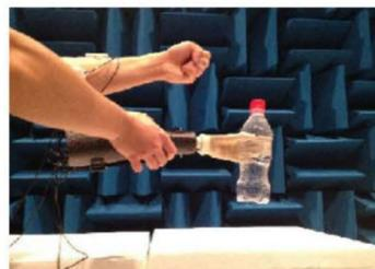
Fig.2 Myoelectric artificial hand system for emission measurement
